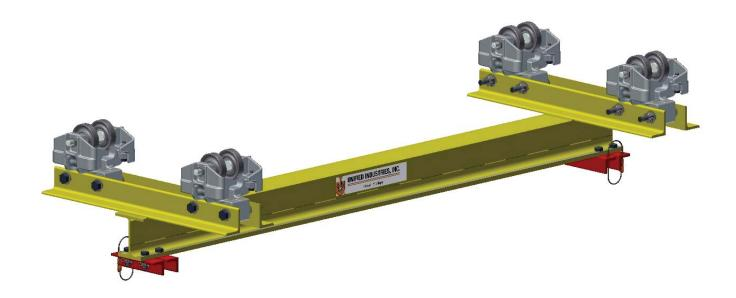
**Unified** light load bridge cranes are designed for the suspension of portable spotwelding guns, power tools, balancers, hoists, fixtures etc., and other light loads not exceeding 1000 lbs. (454kg).
