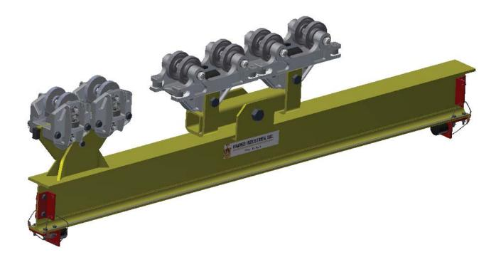
**Unified** heavy duty telescoping self-equalizing tandem trolley units are designed for the suspension of portable spotweld guns, power tools, balancers, hoists, fixtures, etc., and other loads not exceeding recommended rated loads. See next page for rated loads of various extensions.
